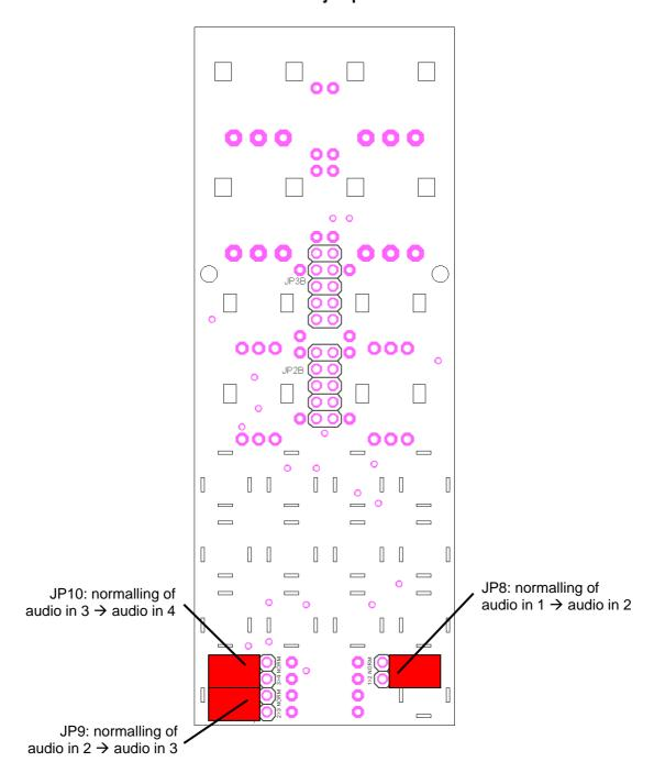
The pin headers JP8, JP9 and JP10 may be used for the normalling of the input signals.
