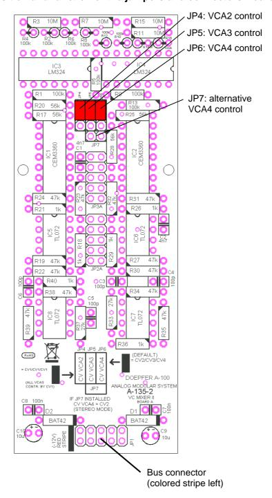
The pin headers JP4, JP5, JP6 and JP7 are used to determine the control voltages for the VCAs 2-4:
