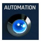
The automation light indicates when the A4-1B hardware is synced and working with the software control plugin inside your DAW or the calibration panel.
