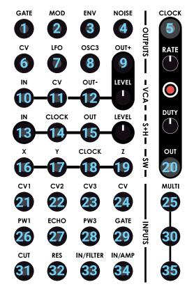
The VCA itself is logarithmic, and near the end of the Level range, you should get a +18db gain, or x10 gain on voltage. Unity gain is at about 3 o'clock. Maximum voltage is +/-10V output.
