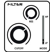
The filter can self-oscillate, starting when the resonance is above 3 o' clock. The sound of the self oscillation will be much different in the 2 filter modes. **HP** has a more agressive sound. The filter has no obvious note tracking, but you can easily achieve that via patching.
