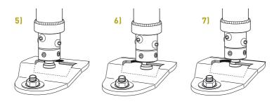
→ Loosen the tightened screw G (Fig. 8) and slide the retaining ring F downwards until it rests on the top of the mounting accessory (Fig. 9).
