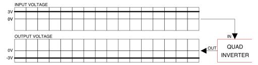
Similarly, if you send a waveform to an input, the output will be an inverted copy of that waveform. This is particularly useful when you want a control voltage (such as an LFO or envelope) to inversely impact the parameter it's modulating.
