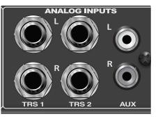
These inputs are for your audio sources (mixer, audio interface, CD player, etc.). Only balanced cables should be used when connecting the balanced TRS inputs of your Central Station to these devices. Because of the Central Station's passive circuitry, using unbalanced cables can reduce the output level and can introduce noise into your system.
