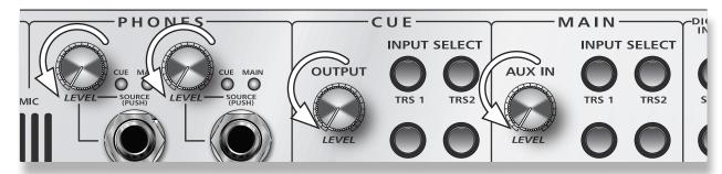
"Zero" the Main, Cue, Aux In, and Phones level knobs by turning them fully counterclockwise. If you have speakers or other gear connected to the Main L/R outputs, turn them all the way down and make sure that the amplifier is powered off.
