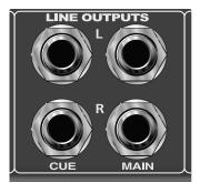
These outputs are ideal for connecting external headphone-distribution systems or external mastering units. Again, only balanced cables should be used when connecting your Central Station to these devices. Because of the Central Station's passive circuitry, using unbalanced cables can reduce the output level and can introduce noise into your system.
