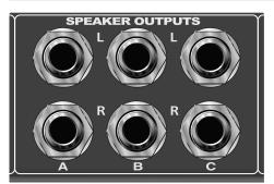
These three stereo pairs of left (L) and right (R), line-level, 1/4" balanced TRS outputs can connect to powered monitors or to power amps for passive speakers. Only balanced cables should be used when connecting the Central Station to your monitors. Because of the Central Station's passive circuitry, using unbalanced cables can reduce the output level and can introduce noise into your system.
