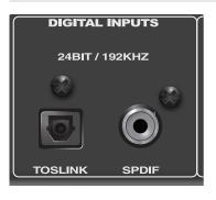
Central Station automatically reads and locks to the sample rate of the incoming digital stream and can receive and lock to sample rates of 44.1, 48, 96, and 192 kHz. Both of these digital inputs are designed for the S/PDIF stereo digital format.
