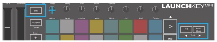
Holding Shift and pressing Arp or Fixed Chord will select the track below or above the current track, respectively. Doing so will also automatically arm the newly-selected Reason track.
