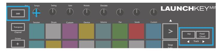
While in Cubase's Mixconsole, hold Shift and press Arp or Fixed Chord to select the track left or right of the current track, respectively. Doing so will also automatically arm the newly-selected track.
