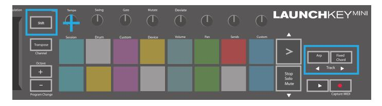
Holding Shift and pressing Arp or Fixed Chord will select the track before or after the current track, respectively. Doing so will also automatically arm the newly-selected track.
