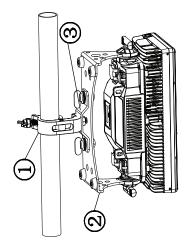
The 32 Hex Panel IP is fully operational in three different mounting positions; hanging upside-down, mounted sideways on trussing, or set on a flat level surface. Be sure this fixture is kept at least 12m (40ft) away from any flammable materials (decoration etc.). **ALWAYS** use and install the supplied safety cable as a safety measure to prevent accidental damage and/or injury in the event the clamp fails.
