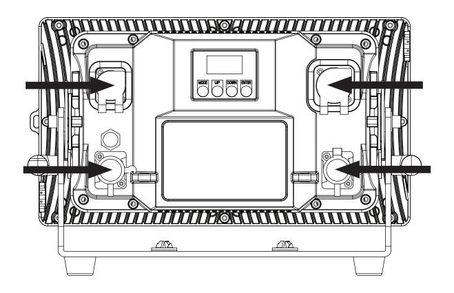
**DMX-512:** DMX is short for Digital Multiplex. This is a universal protocol used as a form of communication between intelligent fixtures and controllers. A DMX controller sends DMX data instructions from the controller to the fixture. DMX data is sent as serial data that travels from fixture to fixture via the DATA "IN" and DATA "OUT" XLR terminals located on all DMX fixtures (most controllers only have a DATA "OUT" terminal).
