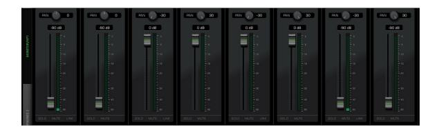
This section contains pan controls, volume faders, and Solo/Mute/Link buttons for each channel of the three 16-channel virtual mixers titled 'Monitor/HP1', 'Headphone 2', and 'Line Out'. 8 channels are visible by default. Click the 'Mixer' switch in Function strip 3 to flip between 8-channel and 16-channel views.
