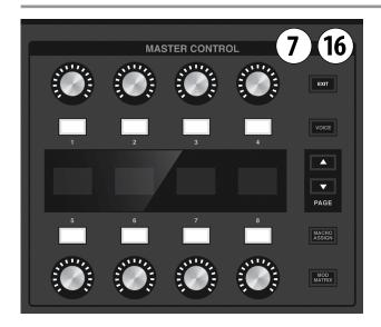
If you like to make your own patches, you might enjoy this top-panel section the most. When a Module is accessed the parameter values are shown in the Right display, selected with the Control buttons, and adjusted with the Control knobs. The Page Up/Down buttons provide access to more parameters whenever a Module offers more than eight. We'll cover the parameters of each Module in <u>Hydrasynth</u> Desktop (p. 24).
