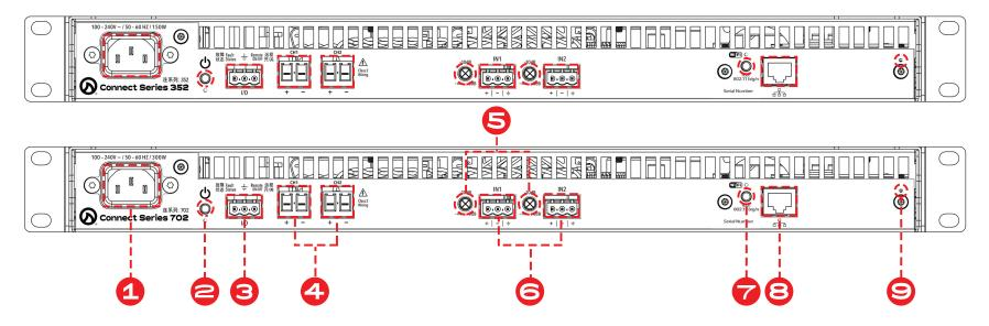
**1. IEC Type Inlet:** For detachable IEC connector. 100VAC-240VAC 50Hz or 60Hz
