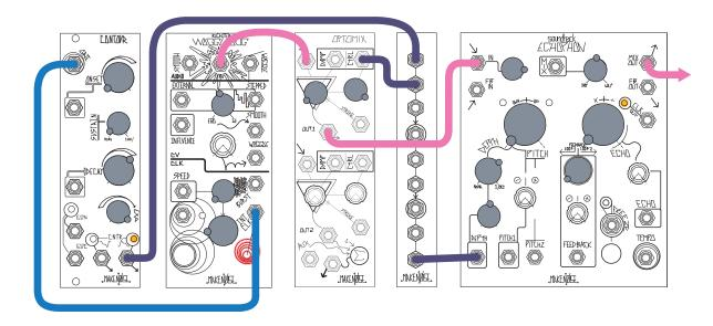
**Sliding Universal Phonogene:** create loops, transpose, maintain original tempo. Depth to 0% (no pitch shift), Mix 5:00, Feedback 12:00 (no feedback)
