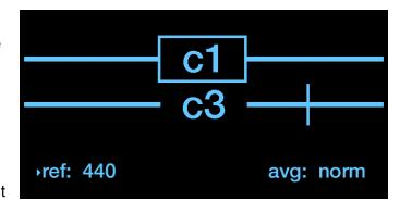
illustration the vertical line is to the right of the note name for CH 2, indicating that CH 2 is playing a C3 ("middle C"), but that the note is sharp.
