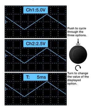
• T: With this option displayed, turning the encoder sets the waveform's time base between 10 s/div and 10 μs/div with seventeen incremental values between these two extremes.
