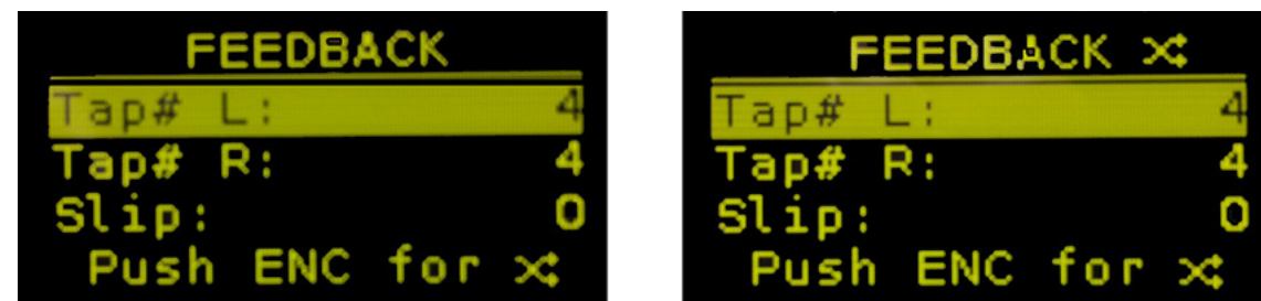
Figure 5. LEFT: The TAP# edit display when Ping-Pong is OFF. RIGHT: The TAP# edit display when Ping-Pong is ON.
