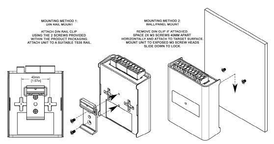
**Note:** The surface mount tabs have been designed to hold the weight of the OCTO only, excess force by caused by cable strain can cause damage.
