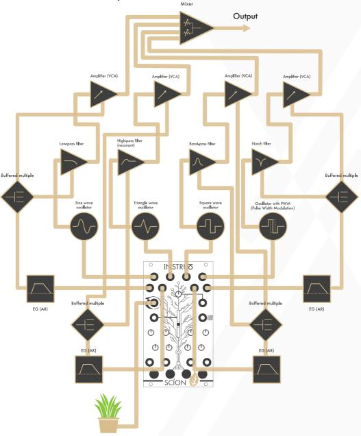
**Summary:** When a biofeedback source is present, the **CV Outputs** send voltages to the oscillators while the **Gate Outputs** trigger the envelope generators. The CV outputs of the envelope generators open the filters and VCAs, allowing the oscillator signals to pass through.
