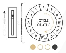
With the **Attenuators** fully clockwise, the OV - 5V output range of the **CV Outputs** will be quantised to semitones.
