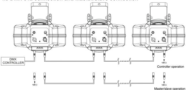
The fixture is equipped with 3-pin XLR sockets for DMX input and output. Only use a shielded twisted-pair cable designed for RS-485 and 3-pin XLR-plugs and connectors in order to connect the controller with the fixture or one fixture with another.
