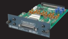
MY8-AD96 8 channel Analog Input Card
