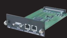
OPTOCORE YS2 16 channel Expansion I/O
