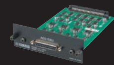
MY8-AE 8 channel AES/EBU format I/O
