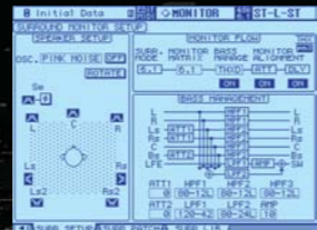
Surround Monitor Setup (THX pm3™ Monitor Flow)
