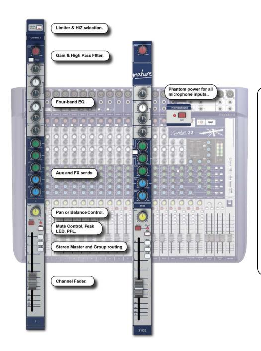
The controls are shown in the order they appear on the console channel strip - from top to bottom. This is not necessarily signal path order. Please refer to the relevant signal path diagram (section 4).
