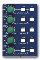
The Aux Master Output channel determines the output level of a whole Aux mix (the sum of all Aux contributions). That is, the Aux 1 Master controls the Aux 1 output level, which is the sum of all Aux 1 contributions from the input channels.
