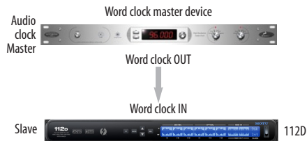
Figure 4-10: Slaving the 112D to word clock. For the 112D clock source, choose 'Word In'.
