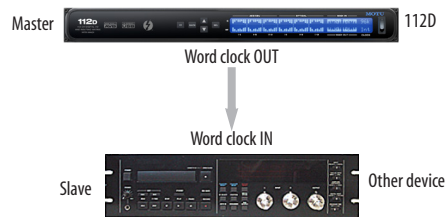
Figure 4-9: Slaving another digital audio device to the 112D via word clock. For the 112D clock source, choose any source besides word clock, as it is not advisable to chain word clock.
