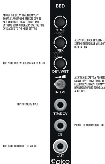
ADJUST FEEDBACK LEVEL! IN FULL CW SETTING THE MODULE WILL GO TO SELF
