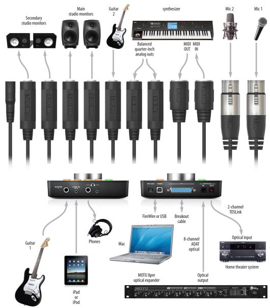
Figure 4-7: A typical Track16 studio setup.
