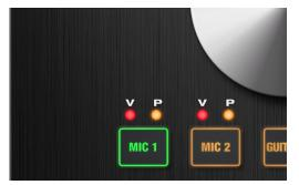
Figure 4-2: The phantom power (V) and pad (P) LEDs for the mic inputs
