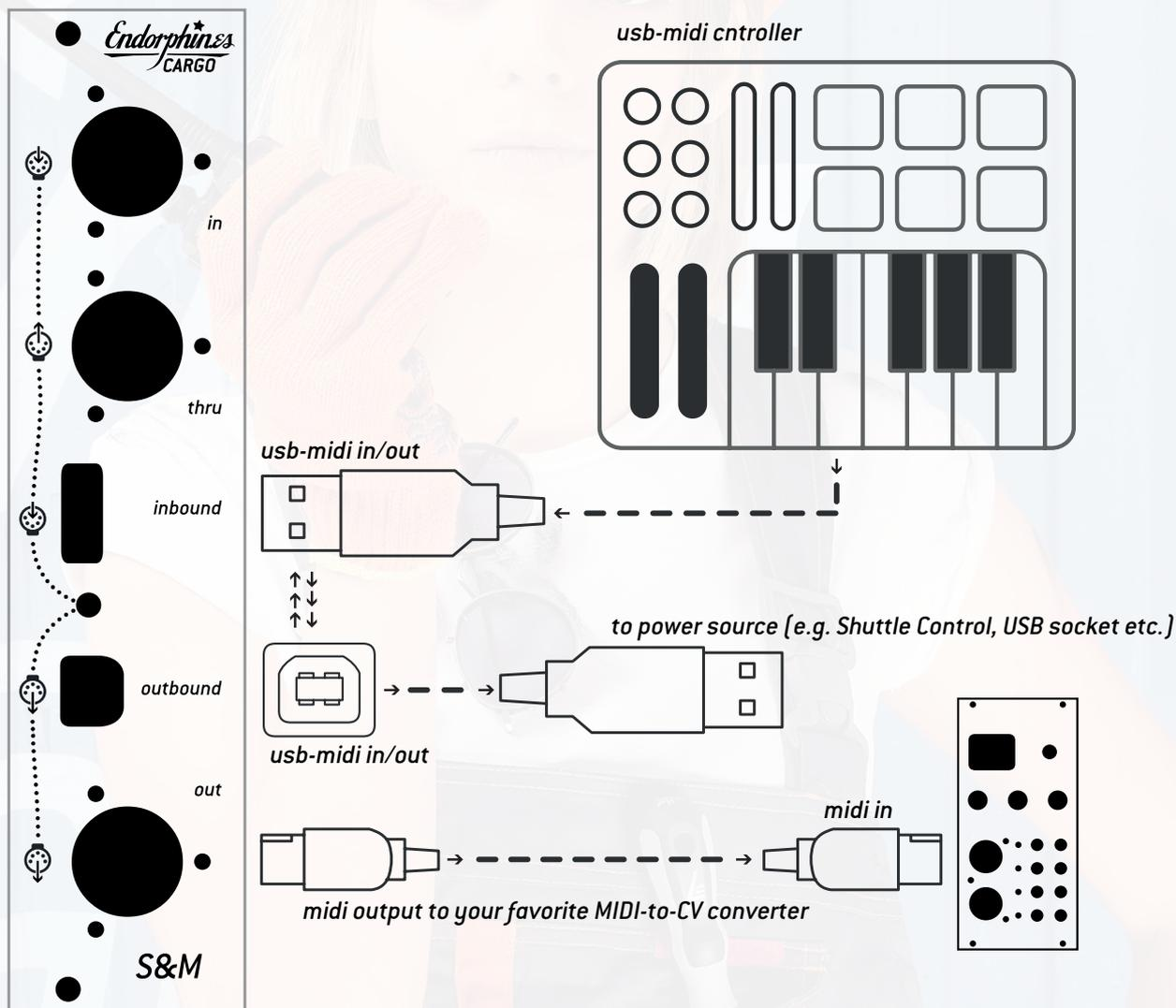
**Usually the Shuttle Mate is powered from USB (via the USB-MIDI OUTBOUND socket) so no extra power supply is required.**
