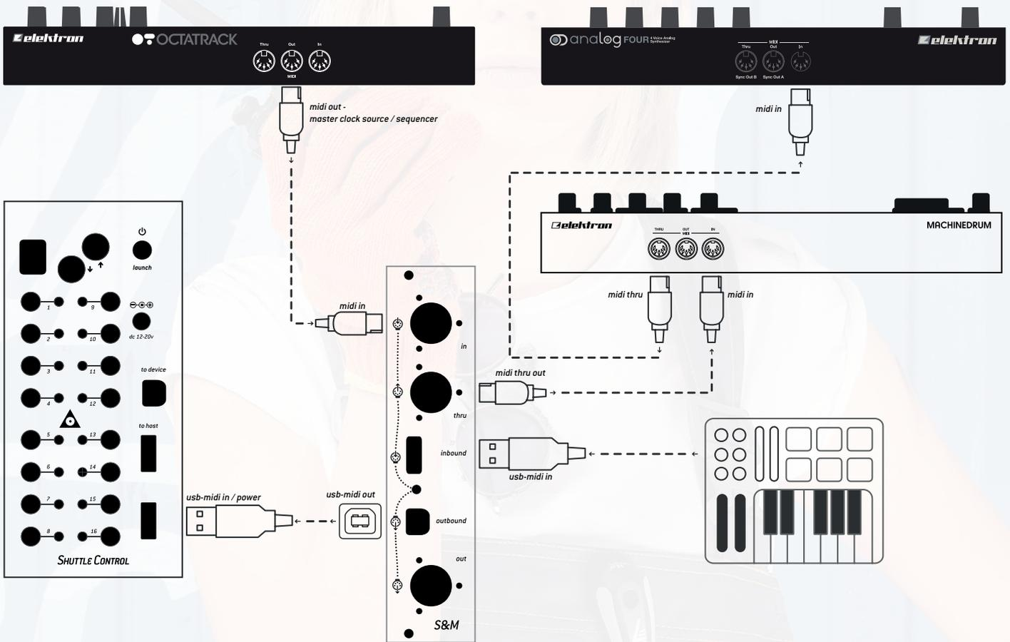
2. **In this setup we use Shuttle Mate as a converter from USB-MIDI into a physical MIDI jack**, which isn't a trivial task especially when you want to avoid using a PC/MAC/iPad during your performance.
