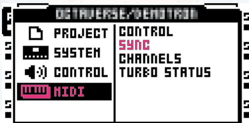
3. Select the checkbox **SEND [X]** in the **TRANSP** section **pressing ENTER (Yes)** and then navigate **RIGHT (>)** with the arrow button **to the CLOCK section** and **press ENTER (Yes)** to choose the **SEND [X]** checkbox.
