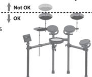
Attach the cymbal rods so that they face straight up, to prevent the drum stand from falling over.
