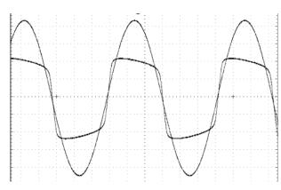
This shows the signal very heavily clipped, virtually to a square wave.
