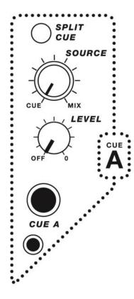
MODEL 1.4 has two independent Cue systems, A and B. Cue A routes to the right hand side headphone monitor and the Cue B routes to the left hand headphone monitor. The dual Cue system makes it much easier for two DJs to perform on the mixer together as each can select a separate channel to monitor without interfering with the other performer's monitoring. This dual system also allows for Cue interaction between two mixers linked together. See page 13 for details of mixer linking.
