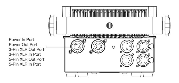
**DMX-512:** DMX is short for Digital Multiplex. This is a universal protocol used as a form of communication between intelligent fixtures and controllers. A DMX controller sends DMX data instructions from the controller to the fixture. DMX data is sent as serial data that travels from fixture to fixture via the DATA "IN" and DATA "OUT" XLR terminals located on all DMX fixtures (most controllers only have a DATA "OUT" terminal).
